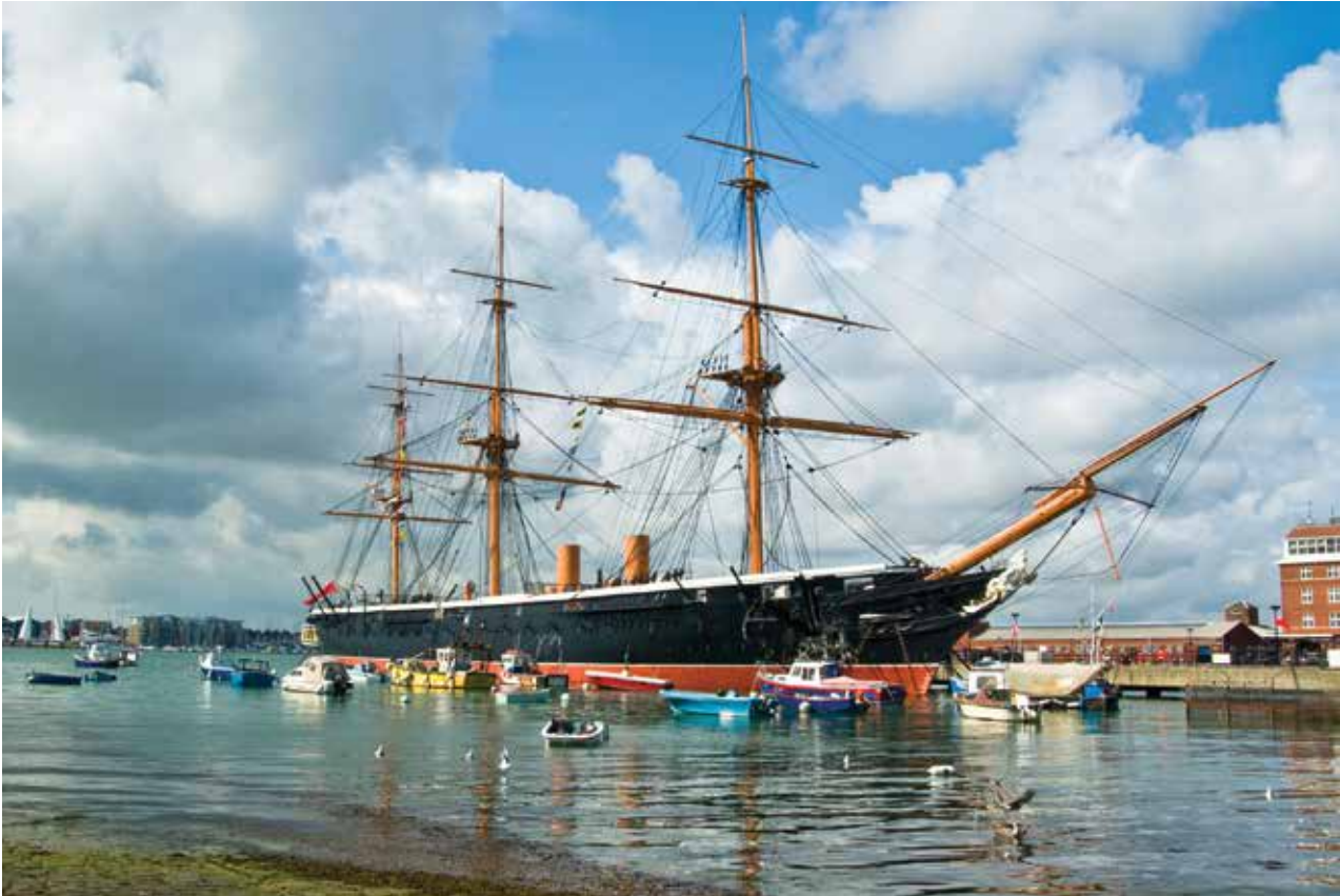
HMS Warrior . Her commissioning was a response to the 1858 launch of France's first ironclad, La Gloire . Warrior 's radical design featured an armoured box that housed the main guns, boilers and engine.
