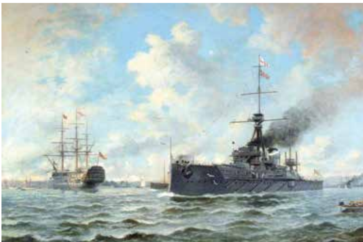
HMS Dreadnaught . Her entry into service in 1906 revolutionized naval power. She was the first capital ship to be powered by steam turbines, making her the fastest battleship in the world at the time of her completion. Painting by H.J. Morgan.
